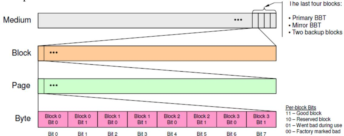
It marks as “Bbt0” in spare area of Primary BBT, and marks as “1tbB” in spare area of Mirror BBT.
